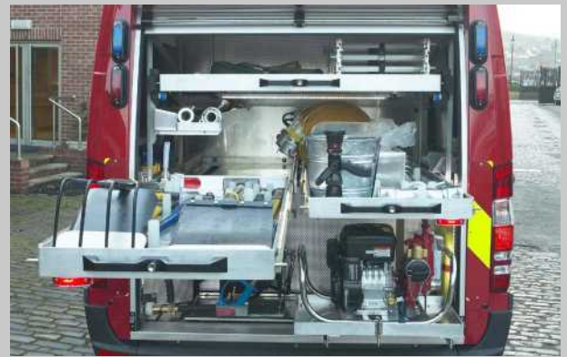
Comprehensive storage facilities with sliding trays, and drawers etc to suit a customer's equipment.
